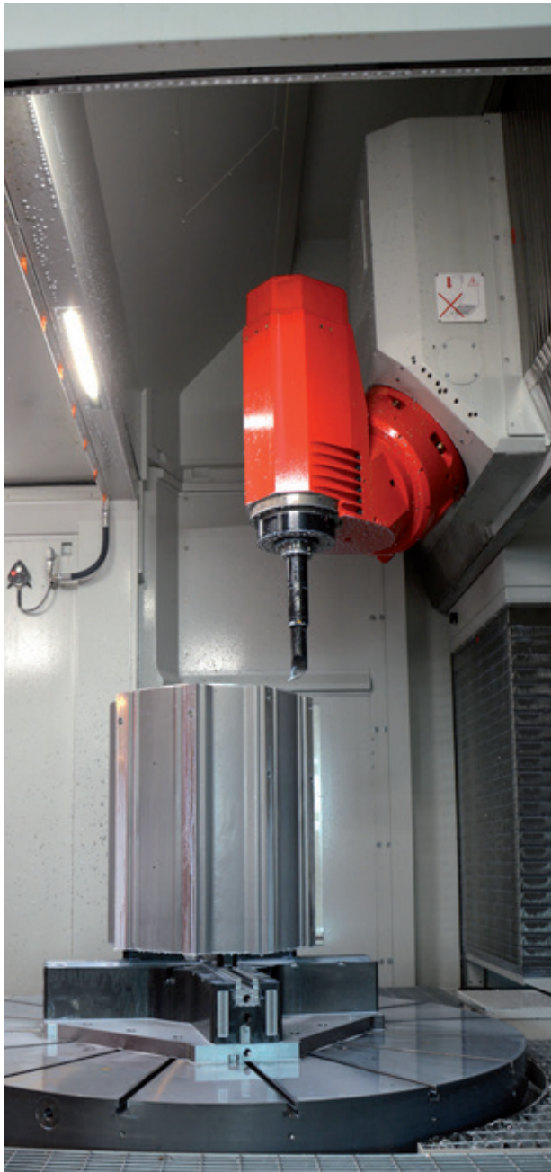
View of the work area of EMCO's Umill 1800, a 5-axis milling and turning machine used by Schwarz Elektromotoren: Reaching rotational speeds of up to 250 min -1 , the NC rotary table is able to machine components in the same way as a vertical lathe. The component shown in the picture is the biggest electric motor housing built by Schwarz so far.
