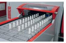
Blank feeding with indexing conveyor
