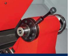
**AUTOMATIC TAILSTOCK** with finely adjustable manual quill.
