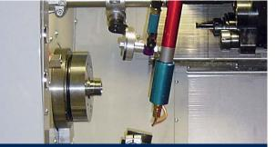
The cold air nozzle can be used for pin-point cooling during dry
