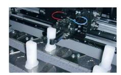
EMCO Swing Loader with raw-part gripper
