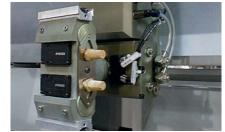
Vacuum suction gripper for fragile blanks
